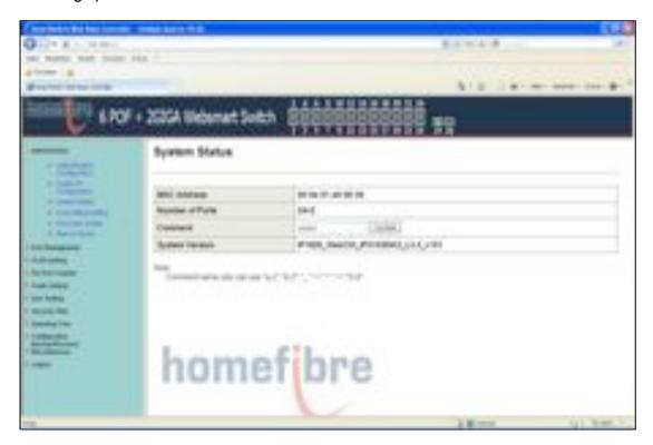
If you want to modify the MAC address of this switch, enter MACIDFix.htm behind the IP address. Example: http://(IP address)/MACIDFix.htm. Please note that this web page is case-sensitive. The web page name should be exactly the same as the web link shown above.
